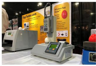
The ORKA egg shell strength tester offers highly accurate readings on the strength of shells. Photo: Jake Davies
